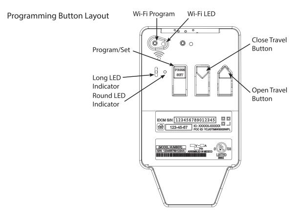
**NOTE**: Each programming step has a 30 second time limit for completion after the function is initiated. After 30 seconds, both LED's will illuminate RED indicating time has expired and the step must be restarted. Restart the step as many times as necessary to complete the programming.
