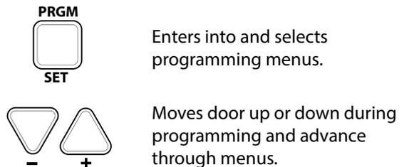
**NOTE:** While setting limits, the powerhead has a 30 second time-out period when none of the three programming buttons have been selected. If you see two solid red flashing LEDs or if the LEDs flash red three times and then go OFF, you have run out of time and must go back to the beginning of the travel limit setting step.
