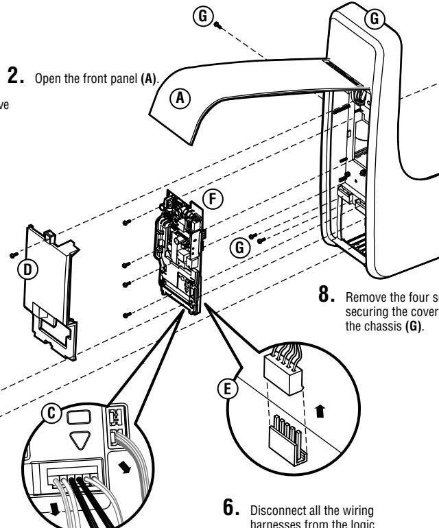
4. Disconnect the wires coming from the safety reversing sensors, door control, door lock and cable tension monitor from the logic board (C).
