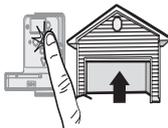
**3** Once the door is in the desired UP position press and release the Adjustment Button. The garage door opener lights will flash twice and the DOWN Button will begin to flash.
