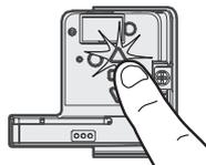
**4** Press and hold the DOWN Button until the door is in the desired DOWN position.
