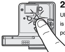
**2** Press and hold the UP Button until the door is in the desired UP position.
