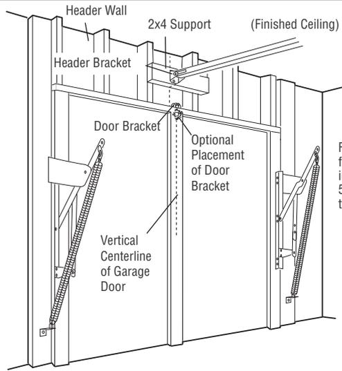
For a door with no exposed framing, or for the optional installation, use lag screws 5/16"x1-1/2" (not provided) to fasten the door bracket.
