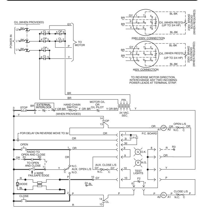
**NOTE:** Terminals R1, R2 and R3 are on optional external terminal block.
