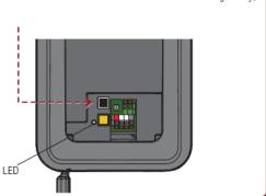
STEP 2: Push and hold the black button until the door reaches the desired UP (open) position.
